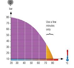
**MAXIMUM WORKING PRESSURE** 40 BAR AT 70°C
